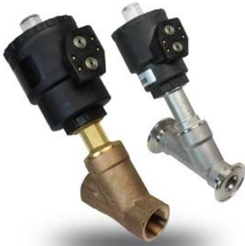
The Angle Seat Valve is a 2/2-way pneumatically actuated piston valve for liquids, gases, vacuum, steam and some aggressive fluids. The superior design of the piston is unique to the market, enabling the plug to retract farther from the flow path, ensuring the highest flow capacity. The dual packing stem seal design (ss models only), and a large diameter self-aligning stem ensure the highest cycle life.
